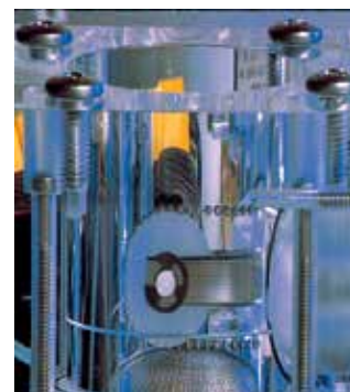
A bed of bronze beads inside the Model 3400A breaks up powder agglomerates before dispersion.
